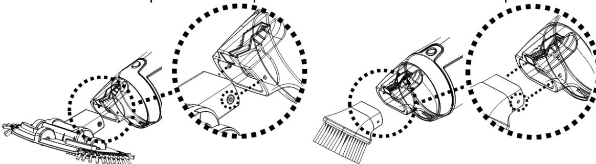
NOTE: To replace the brushes on the suction head, lift one end and pull the brush out to make space for a new one.
