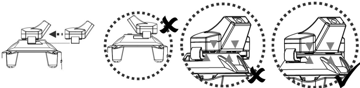
2. Plug the female jack of the external adaptor into the charging port at the end of the charging base.
